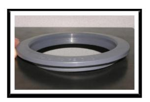
Press the gasket gently into the tubesheet hole by hand, it will self-center and seat. A properly installed gasket will have no deformations around the ID of the gasket, and the top flange will be flush against the top of the tubesheet.
