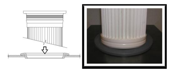
Once the filter is lowered all the way into the gasket, the final sealing of the filter into the gasket will require slow, firm pressure to seat the stepped top down into the gasket and kick out the bottom flange to engage the seal. Stepping on the filter top is acceptable as long as steady, even pressure is applied.
